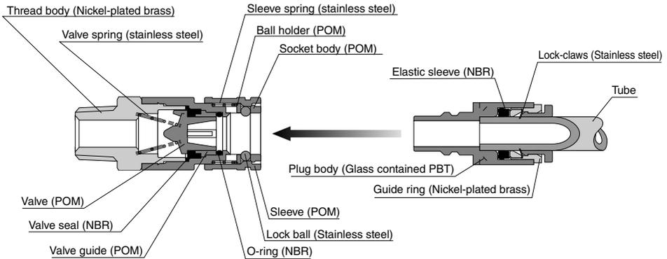
※ The above figure is the construction of 15 series. E3 and E7 of 20 series have different construction and materials from 15 series.
