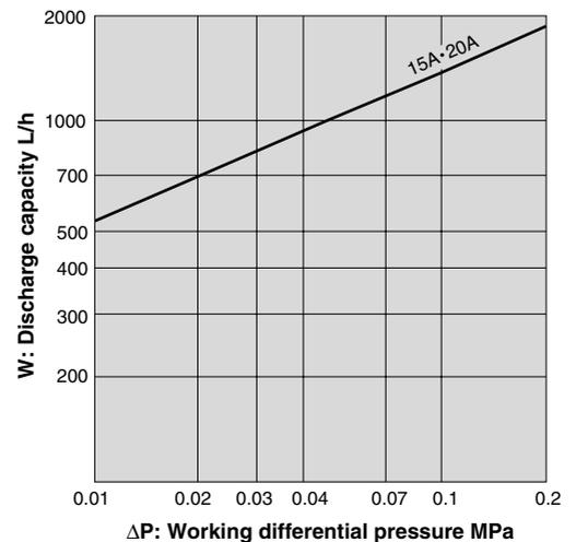
• This chart shows the maximum discharge. In designing a system, set a sufficient safety factor (two or three times).
