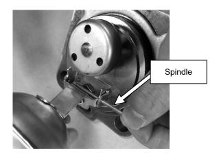
[Procedure 3] Remove the split pin from the cock. With fixing the cock (width across flat: 9 mm), remove the nut by using spanner (width across flat: 22 mm), and then remove the collar and the name plate.
