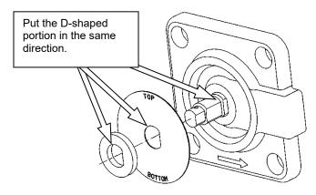
[Procedure 4] Connect the float holder and float (P) assembly with the spindle. Check that the float (P) assembly moves smoothly, and that the seat surface of the valve is in contact with that of the valve seat.
