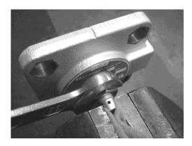
[Procedure 4] By pulling out the cock from the cover, the cock assembly can be replaced.
