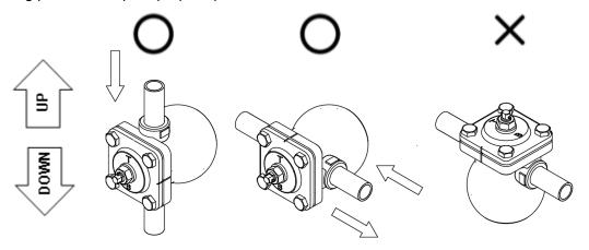
\* Allowable tilt from horizontal line is within ±10°.
