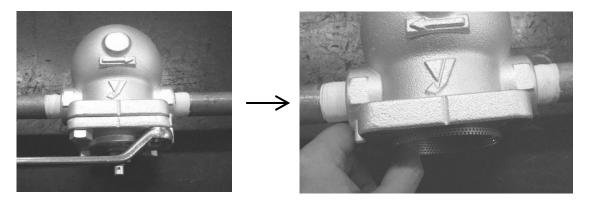
[Procedure 2] Pull out the spindle from the float holder and remove the float (P) assembly.
