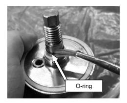
[Procedure 2] Attach the cock (after taking Procedure 1) to the cover. Check that the cock gasket (P1) is attached to the cock properly. If not, it may cause steam leakage to the outlet side.
