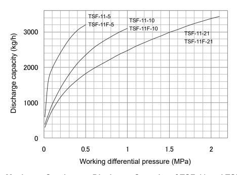
Maximum Continuous Discharge Capacity of TSF-11 and TSF-11F
