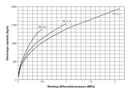
The discharge capacity shown on the above chart is the maximum value. In designing a system, select a steam trap with a sufficient safety factor (more than two times the regular level).
